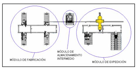
A lot of final degree projects have been carried out with this manufacturing cell, working over the stations communication. This communication is carried out through a Fipway net that subsequently, by means of the Premium and Micro of Modicon Telemecanique automatons, is controlled with the help of PL7pro software.
