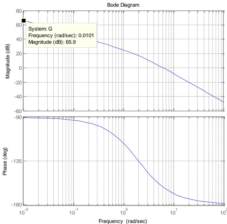
$$20 \log |G(j\omega_0)| = 20 \log K - 20 \log \omega_0 = 20 \log K - 20 \log 0.01 = 20 \log K + 40 = 66 \text{ dB}$$
